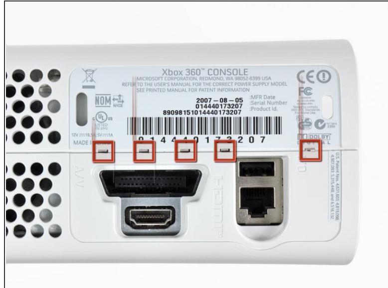
ⓘ The upper and lower cases are held together by seven release latches located on the back of the console. Their locations are highlighted in red.
