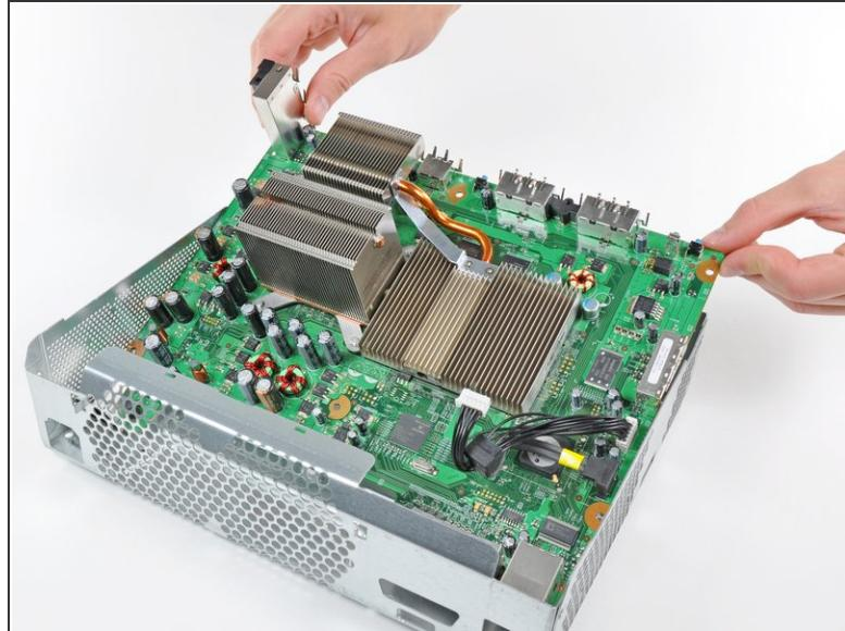
**i** Turn the Xbox over, being careful not to let the motherboard fall out of the chassis.
